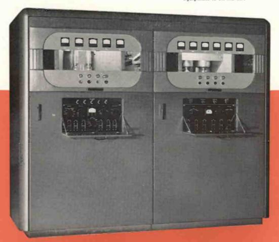
The Collins 737A 5 kw FM transmitter consists of two basic units, a type 732A 1 kw exciter unit, and a 5 kw grounded-grid power amplifier, plus an external air-cooled plate transformer.
