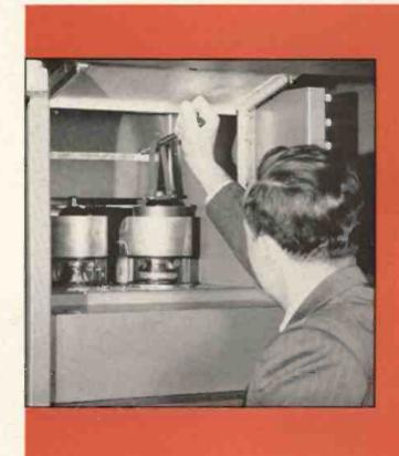
The power amplifier output tubes are also easy to remove with accessory equipment which is furnished with each of the transmitters.
