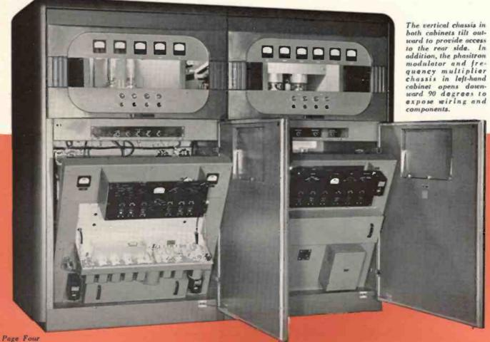
and power amplifier cabinets. Master power controls provide step by step or automatic sequencing control of the entire transmitter operation.
